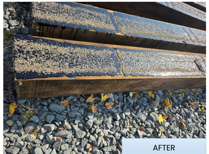
Figure 4. Before and after pictures of Tietan with aggregate applied hot to several bridge ties.
