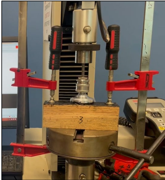
Figure 1. Left - Sample clamped into place prior to pull-adhesion testing. Aluminum dolly was adhered to the Tietan surface using a strong epoxy adhesive. Right - Representative Pull-Off Adhesion Data collected from Tietan Bonded to treated wood tie specimen. Pull rate was set at 5 mm/min.
