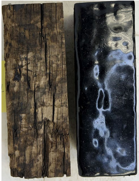
Figure 5. Top down picture of 3"x3"x9" pieces of used railroad ties cut from the same piece of used railroad tie. One is uncoated and the other is coated with an aggregate-free version of the Tietan product.
