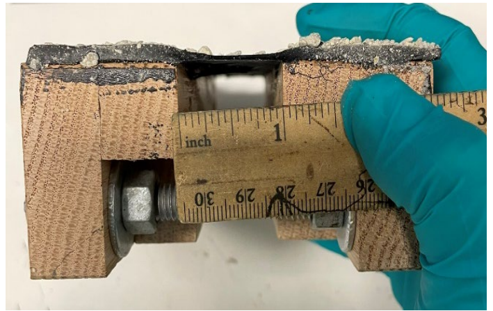
Figure 3. 1/8" Tietan layer as applied (left), and after spreading block to 1" separation (right).
