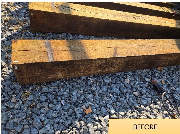
Figure 4. Before and after pictures of Tietan with aggregate applied hot to several bridge ties.
